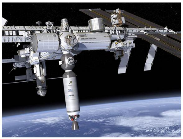
Source: NanoRacks 2016. Figure C-4. Station Module Built from Refurbished Centaur Upper Stage Attached to ISS
